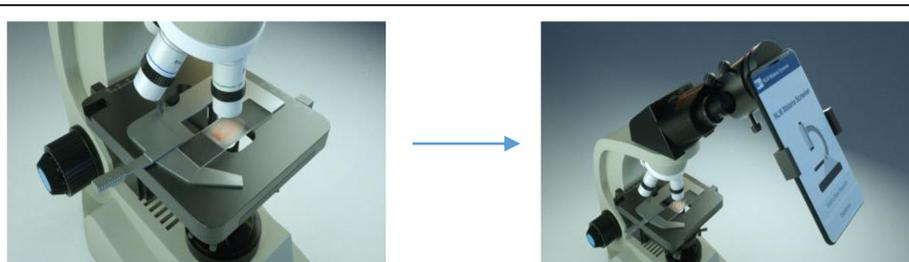
**Fig. 1** System Setup for Malaria Screener. During the (semi-) automated\* screening process, the body of the smartphone is attached to an adapter. The adapter holds the phone, and aligns its camera with the eyepiece of the microscope. \* The system is semi-automated in that the user needs to move the slide manually to search for an ideal field of view while capturing smear images
