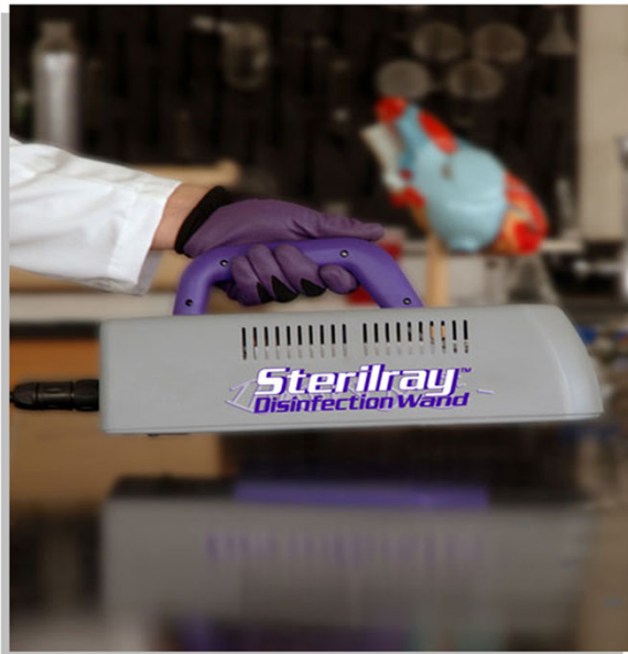
Figure 1 Picture of the Sterilray™ Disinfection Wand far-ultraviolet radiation device. The portable device includes a disinfecting wand weighing 4 pounds attached to a wheeled power pack. The radiant dose (mJ/cm 2 ) of far-ultraviolet irradiation is dependent upon the amount of time and the distance the device is held from the surface being treated.
