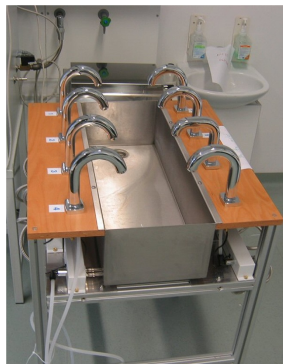
Figure 1 Laboratory set-up of non-touch sensor fittings on a mobile water sink.
